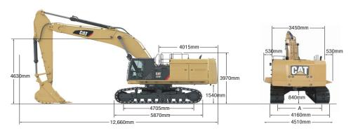
A Track Gauge – retracted 2750 mm
